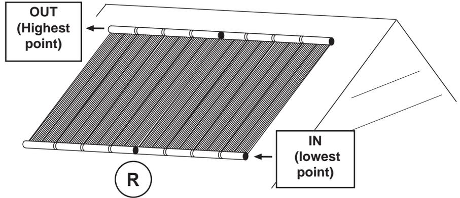
Do not be tempted to use domestic waste pipe, it has not been manufactured to accept the water pressure that is produced by your filtration. Never connect the Poolsolar to a mains water feed. Solar collectors have been designed to receive up to 1.5 bar. Pool filtration is typically +/- 1 bar.
