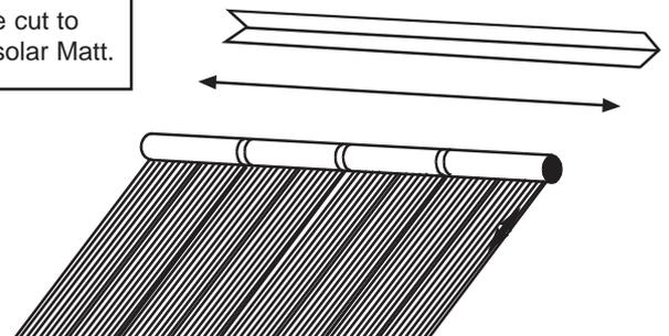
(H) Apply the support angles directly to the roof tiles using liberal amounts of 'roof fixing adhesive paste' (available from your dealer).
