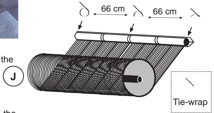
**STEP 8** Apply an adhesive (K) bead every 50 cm to the roof structure and unroll the Poolsolar matting. It is also a good idea to apply adhesive down the very edge of the matting (L).
