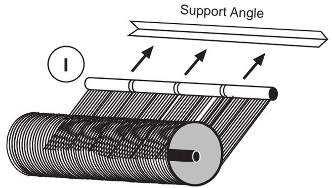
Using the electrical a tie-wraps provided (J) connect the header to support angle every 66 cm.
