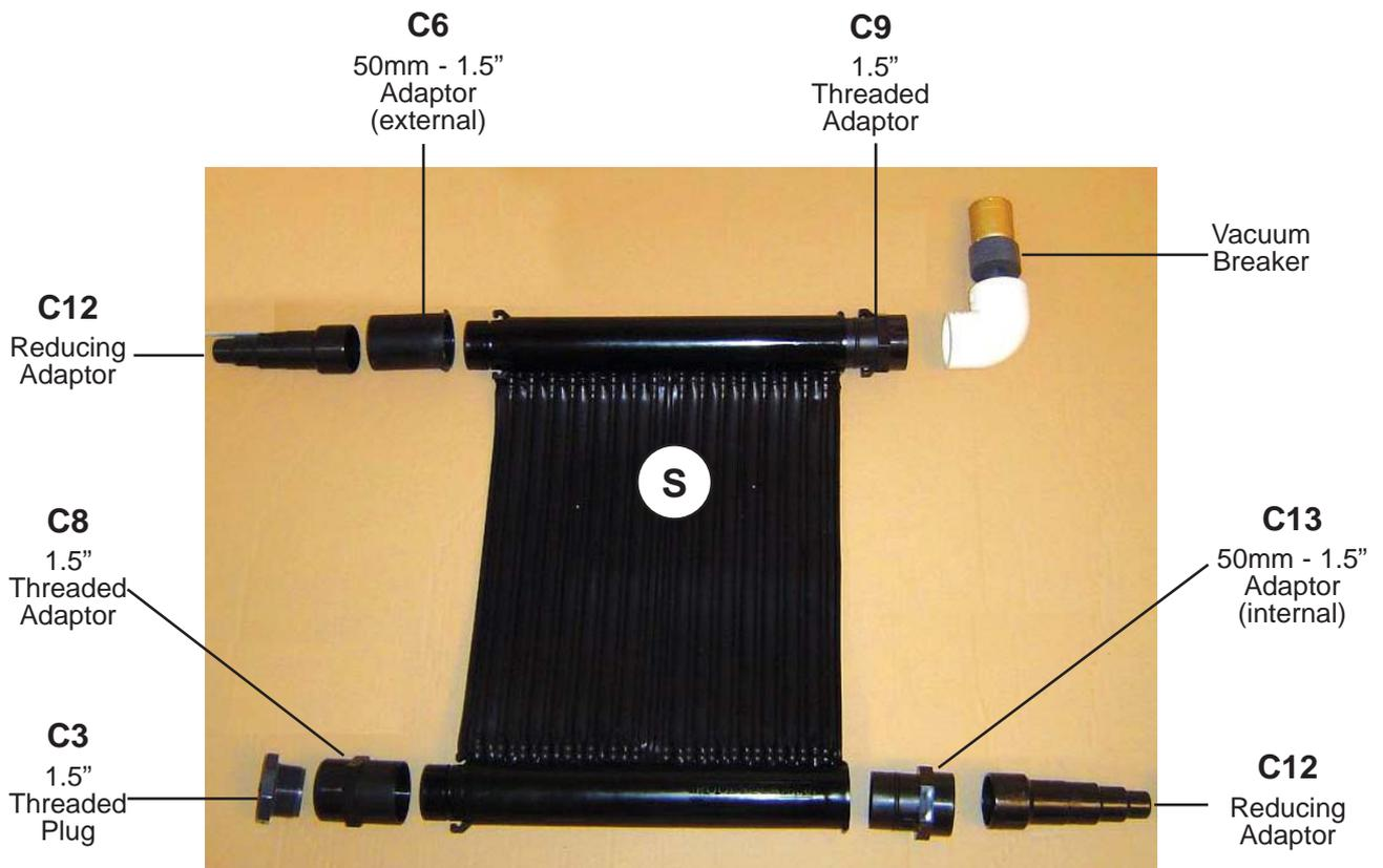
**STEP 11** (T) Insert the correct plumbing adaptors to each corner C6-C8-C9-C13 (See page 8). Glue imperial reducing adaptors (C12) onto plumbing adaptor (C6 & C13) and cut to desired diameter. For all threaded fittings, apply PTFE. tape.
