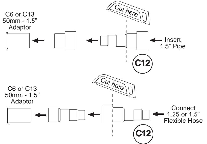
**STEP 12** Connect ABS/PVC 1.5" plumbing to Poolsolar as per diagram below. You will need to install a 3-way valve, this will enable you to direct the water flow to the heater and back to the pool. A vacuum breaker will also be required on solar heating that is 4m or higher above ground level. Vacuum breakers are not required for low level installations. Once all of the plumbing connections have been made, proceed to step 13.
